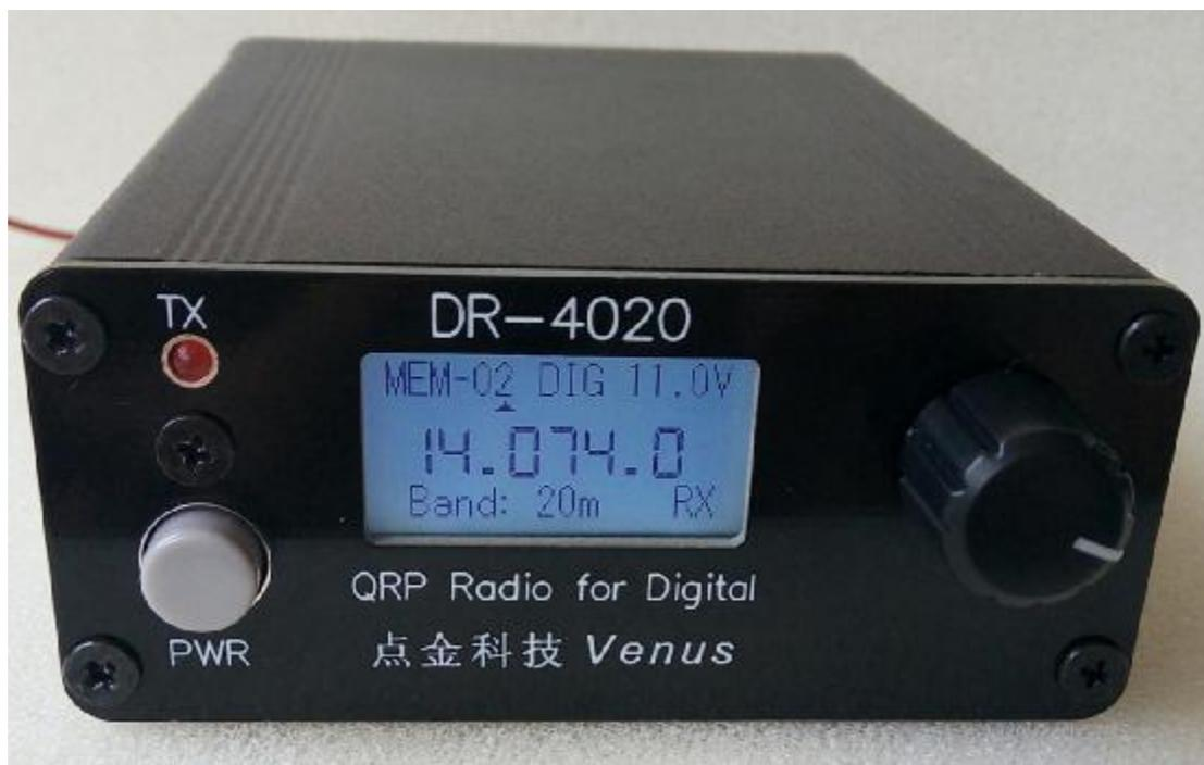
DR4020 is a 40m/20m dual-band radio for digital modes that requires a computer with specific applications to use. It can be used in the popular FT8, FT4, JT65, as well as PSK31, SSTV and other modes.
